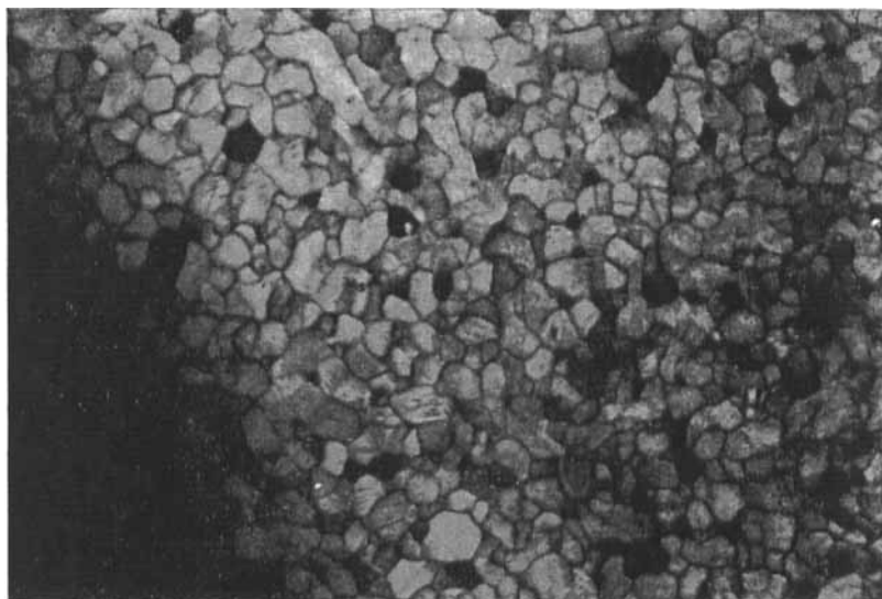
Figure 11. Clear mosaic "phase" of (-)-2-methylbutyl 4-( p -methoxybenzylideneamino)cinnamate passing to the amorphous, isotropic liquid on the left hand side ( \times 37 ); crossed polars.
