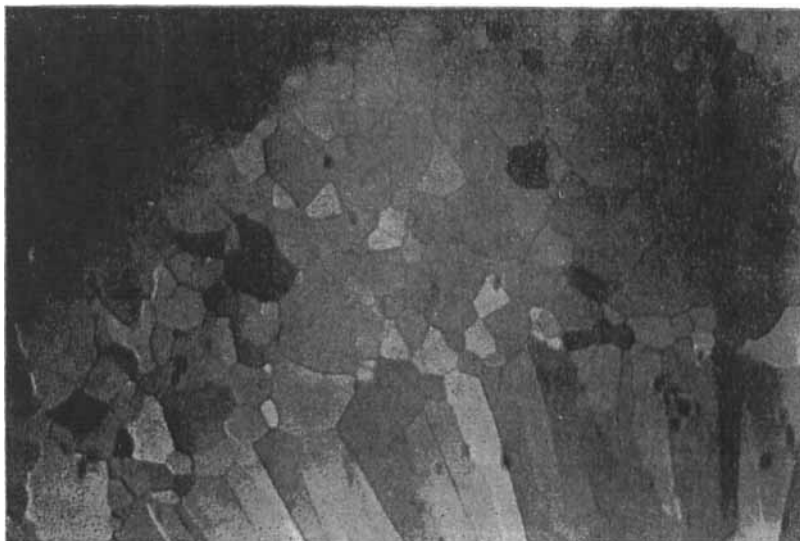
Figure 5. The transition from the "focal-conic" texture of the cholesteric mesophase (lower left hand corner) of di-(-)-2-methylbutyl terephthalylidene-bis- p -aminobenzoate to the blue + green "phase" ( \times 37 ); crossed polars.
