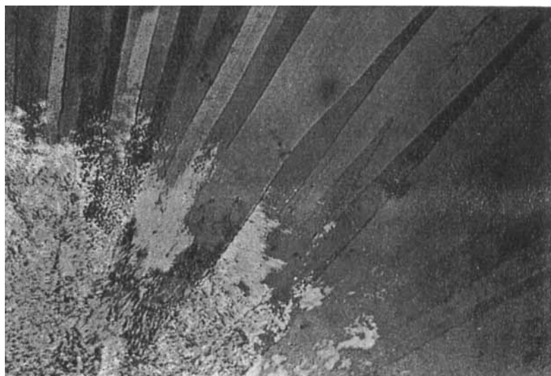
Figure 6. Transitions from the blue + green "phase" of di-(-)-2-methylbutyl terephthalylidene-bis- p -aminobenzoate—lower semi-circle—to the blue isotropic "phase"—seen in the black and white photograph only as a milky band surrounding the semi-circle—to the amorphous isotropic liquid—top left and right hand corners ( \times 37 ); crossed polars.
