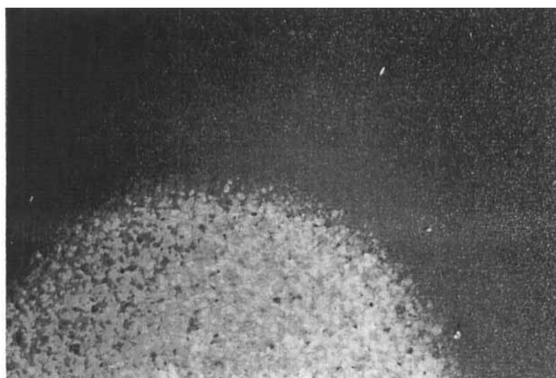
Figure 8. Stripes or blades of the blue + green "phase" of di-(-)-2-methylbutyl terephthalylidene-bis- p -aminobenzoate showing saw-like edges. The "focal-conic" texture of the cholesteric phase is forming in the lower left hand corner ( \times 37 ); crossed polars.
